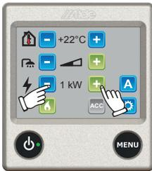
1. Use the + or - button to switch on the electric heating and toggle between the various power modes (Off, 1 kW, 2 kW or 3 kW) The set value will be displayed on the screen. The activated mode is indicated by the + button changing colour to green. If a \*load monitor is installed and set, the boiler will not use more electricity than it is capable of even if 3 kW is selected.
