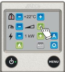
3. More hot water. If you need more hot water, the water temperature can be temporarily increased to around 70°C. Press the "+" button so that the symbol shows fully shaded (black). The boiler returns to normal operation after 30 minutes.
