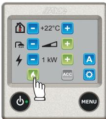
1. Start gas operation by pressing the LPG flame symbol. The LPG symbol is activated and changes colour to green.
