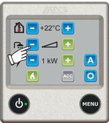
1. No hot water. If domestic hot water is not needed, press the "-" button (symbol becomes empty).
