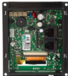
Alternative 2 Rear of panel 3020 HE and 3020, with black sockets.
