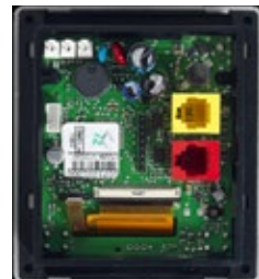
Alternative 3 Rear of panel 3020 HE, with yellow/red sockets.
