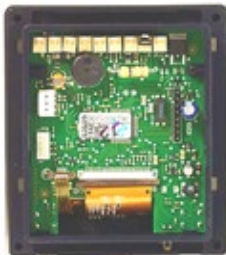
Alternative 1 Rear of panel 3010, without black, red or yellow sockets.
