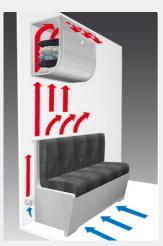
• This is how it should be when the hot air from the convectors flows up behind the sofa and upper cabinets.
