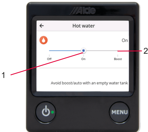
Fig. 8, Hot water production settings
