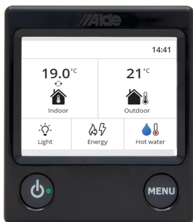
Fig. 12, Single zone start screen, with AC (optional) installed.
